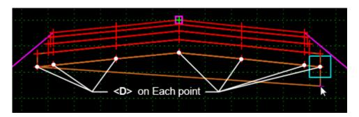
The next steps build the bottom of the subbase. The points are placed in the approximate location. There final position is set by editing the point constraints.
