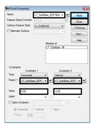
16. Repeat steps 8 through 14 for the remaining points across the bottom of the sub-base component.
