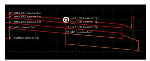
12. Drag and Drop the section onto the RT\_HMA\_Lift1\_Laneline-Top1 point.
