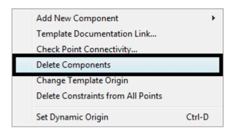
7. <D> and hold, then draw a line through the curb, sub-base, and end conditions components on the right side of the template as shown below. Release the mouse button to complete the delete.
