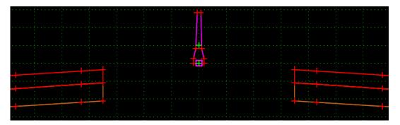
Now the pavement edges need to be attached to the barrier. This is done by modifying the constraints for the those points.
