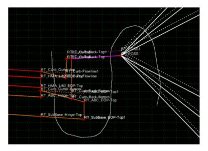
The exposed points still have names used by the curb and gutter component. These must be changed to reflect the new role of the point.
