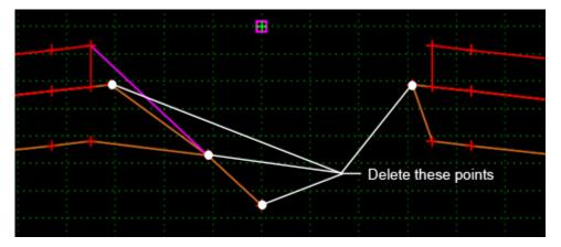
Place a Type-7 barrier in the template. In this case, the center bottom of the barrier is placed on the template origin.
