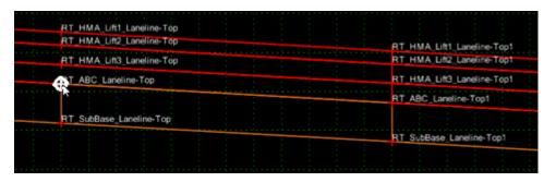
40. <R> on the vertical line between RT\_ABC\_Laneline-Top and RT\_SubBase\_Laneline-Top and select Merge Components from the menu.
