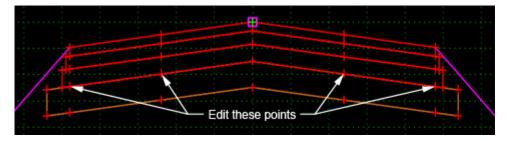
**Note:** The two outside points (HMA\_Lift3\_EOP-Bottom and ABC\_EOP-Top) do not need to be modified. This is because they are built with Vector/Offset constraints which keeps them in line with the other points on that row.
