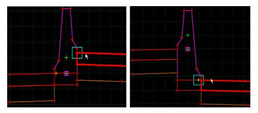
**Note:** This barrier has both a variable height *and* a variable width. If the height is 34" or less, the base is 23" wide. As the height increases above 34" the base varies from 23" to a maximum of 26.75". The maximum height is 40".
